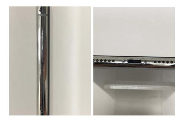
DISQUALIFY SAMPLES Scratches on glasses; Deep scratches on housing
